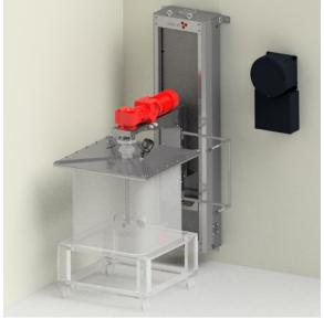
one separation Safe zone separation takes place via a lid with axial compensator including connection for a customer-side extraction system for generating a vacuum in the vessel
