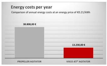
Comparison of the existing agitator and the new VISCO JET® agitator solution
